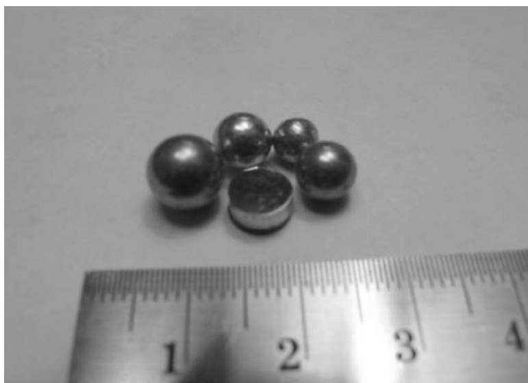
Figure 4.14. Cu spheres with nanocrystalline microstructures prepared by combined liquid-nitrogen temperature and room-temperature milling.
