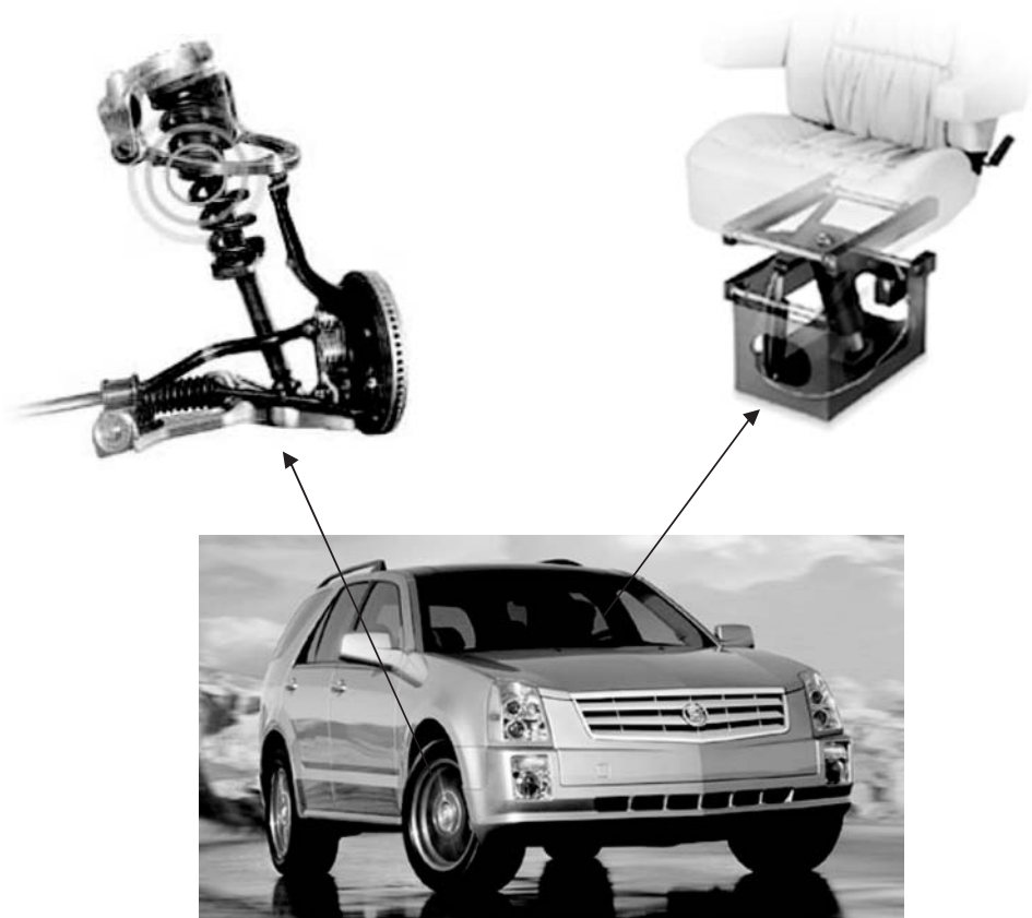
Figure 7.7. Tunable suspension systems using ferrofluids in various sections of an automobile.
